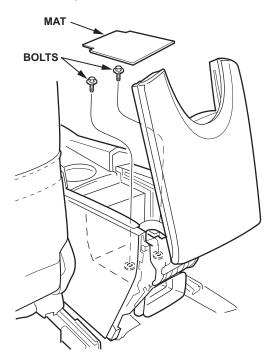
3. Remove the two bolts securing the rear of the center console.
