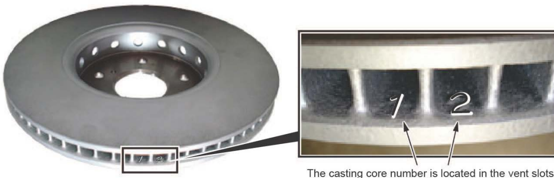
The casting core number is located in the vent slots.
