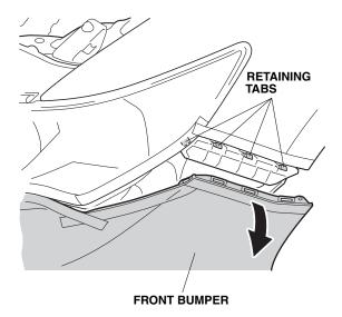
With the help of an assistant, release four retaining tabs on each side.
