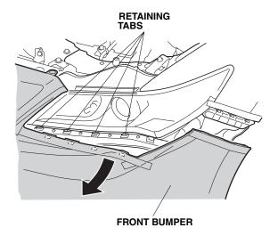
With the help of an assistant, remove the front bumper (unplug the vehicle connector, and release five pins). Place the front bumper on a blanket to prevent damage.
