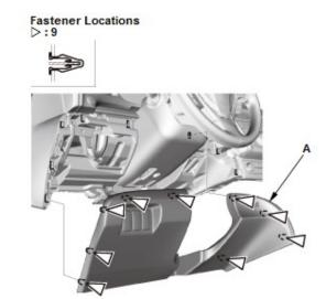
Remove the driver's dashboard lower cover (A). To avoid whitening the dashboard cover at its clip bosses, start by gently and evenly pulling out on the lower edge of the cover to release its lower clips, then work your way up the cover to release its middle and top clips.
