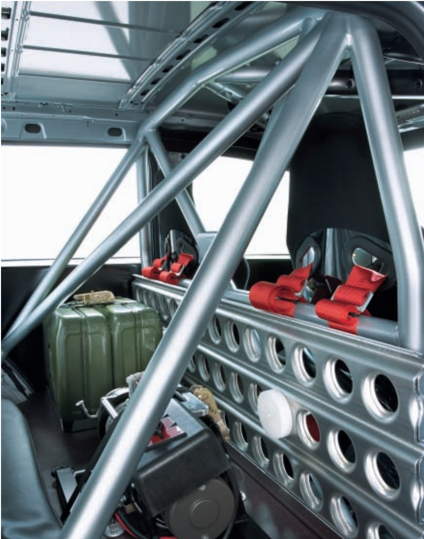
Solid safety cage in the interior
