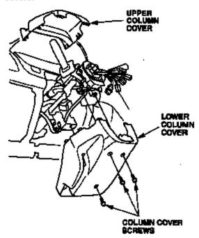
13. 2001–02 models: Unplug the SRS main harness 2P connector, and then detach the dashboard wire harness 4P connector from the cable reel. Remove the screws from the cable reel, and then remove the cable reel from the column.
