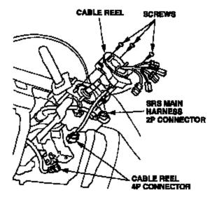
2003 models: Unplug the SRS main hamess 4P connector and the dashboard wire hamess 5P connector from the cable reel 4P and 6P connectors. Release the tab, and then remove the cable reel from the column.
