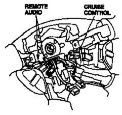
2003 models: Unplug the connectors from the hom, remote audio, and cruise control switches.
