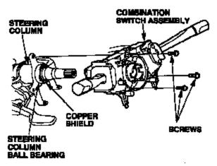
Use a small, flat-tipped screwdriver to lightly dimple the shield in eight places as shown.
