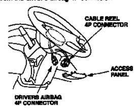
NOTE: When unplugged, the driver's airbag connector is automatically shorted.
