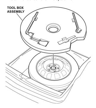
15. Install the spare tire anchor onto the tool box. Make sure the spare tire anchor shows TEMPORARY TIRE towards the handle. If it does not, release the two retaining tabs and flip the anchor to the correct orientation.
