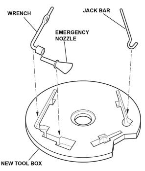
14. Install the tool box over the spare tire.
