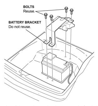
9. Install the new battery bracket reusing the four bolts removed.
