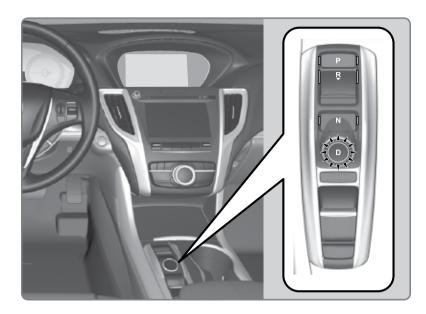
In freezing or sub-freezing conditions, the electronic gear selector response may be slow. Always apply the brake pedal before shifting into Park (P), and confirm that (P) is shown on the gear position indicator before releasing the brake.
