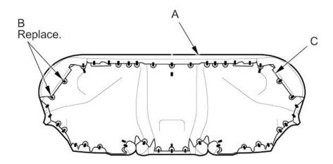
3. Pull back the edge of the seat cushion cover (A) all the way around, and release the upholstery rings (B). Release the hooks (C) of the lateral wires (D) from the longitudinal wires (E) on the pad, then remove the seat cushion cover.
