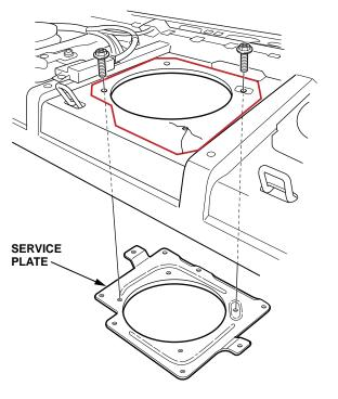
19. Using a felt tip pen, mark the eight holes in the service plate to the rear shelf to be drilled.
