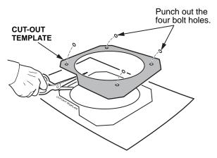
15. Lay the paper template down on the top of the rear parcel shelf and install two bolts in a cross-diagonal location as shown.
