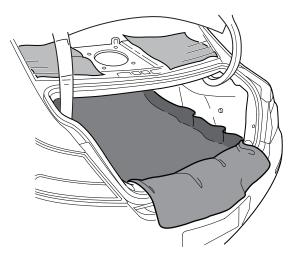
14. Cut out the paper template provided in the kit. Punch four holes in the template where the subwoofer mounting bolts go through.
