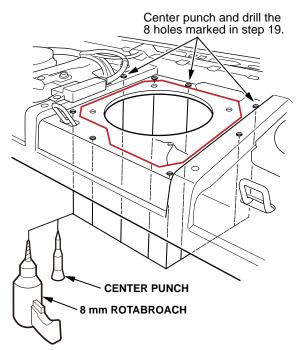
22. Using an 8 mm diameter Rotabroach, drill the eight holes marked into the underside of the rear shelf.
