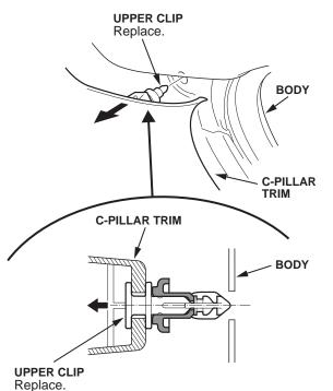
9. Pull the C-pillar trim by hand to detach the clips to release the hooks, then pull out the trim from the rear shelf.
