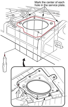
SERVICE PLATE ATTACHED TO THE UNDERSIDE OF THE PARCEL TRAY
