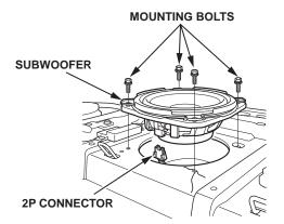
12. Disconnect the 2P connector, and remove the subwoofer.
