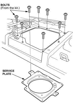
27. Torque the eight service plate bolts to 6.9 to 11.9 N•m (5 to 8.8 lb-ft).
