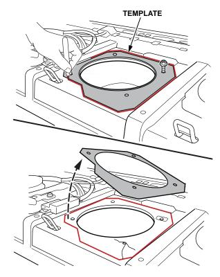
17. Inspect the rear shelf for cracking that may extend past the cut line. If any crack extends beyond the cut line, drill an 1/8" hole into the end of the crack. Fill the hole and crack with J-B Weld.
