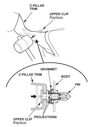
8. Pull back the top of the C-pillar by hand to remove the upper clip from the body.
