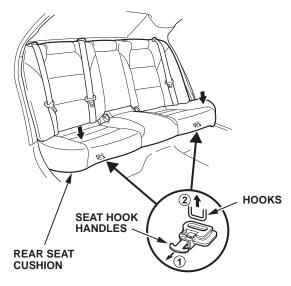
2. Remove the seat cushion, and release the center seat belt buckles from the slits.
