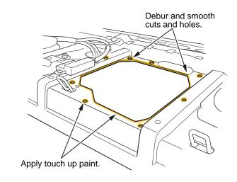
25. Use touch-up paint to coat the newly cut area, drilled holes, and any area where J-B Weld may have been used to prevent rust from occurring.
