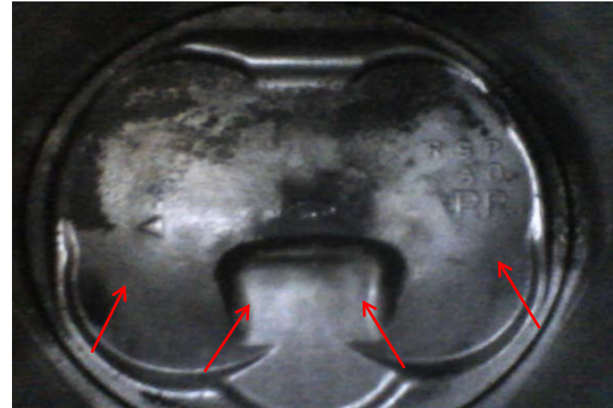
Good: Example of a 2015 1.5L L4 (direct injection) with 20,000 miles and no oil problems. Piston top has a clean area.
