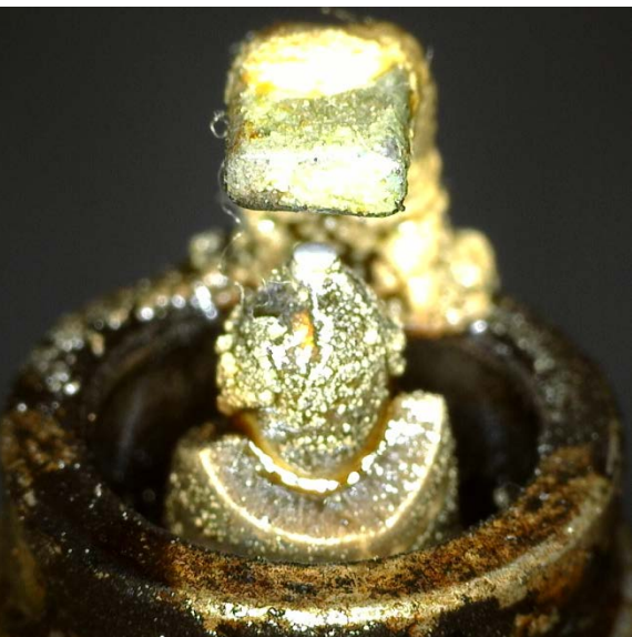
No good: Insulator badly broken
