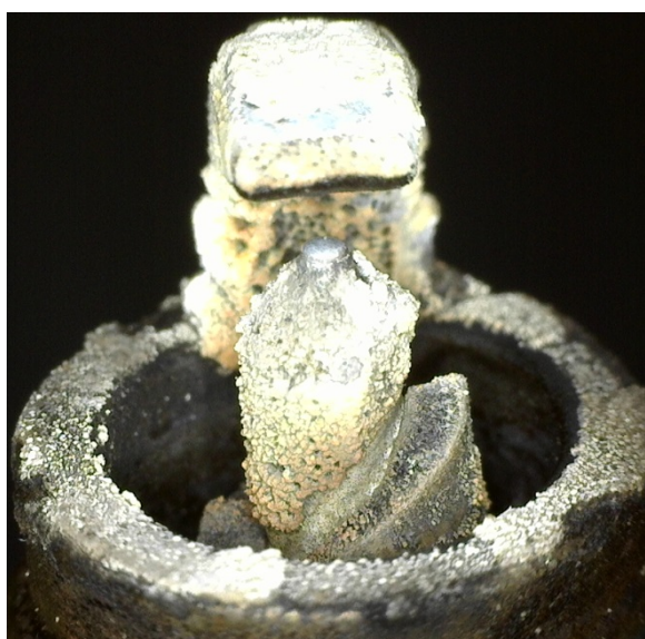
No good: Insulator badly broken
