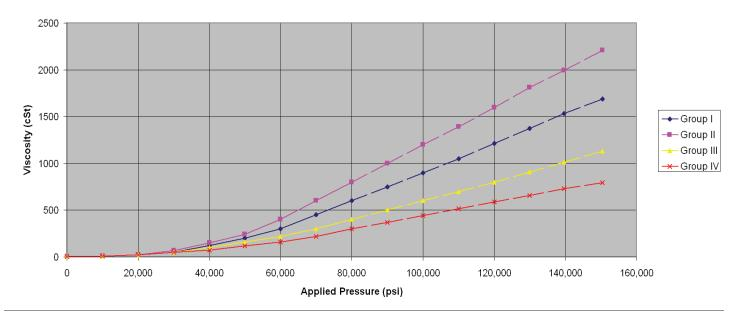
figure 4 - Oil Viscosity Change with Applied Pressure
