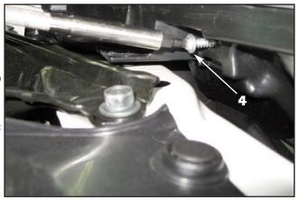
4. Pull the top of the factory grille towards you. Use a torx T-20 tool to remove the eight (8) torx screws holding the center section of the grille in place.
