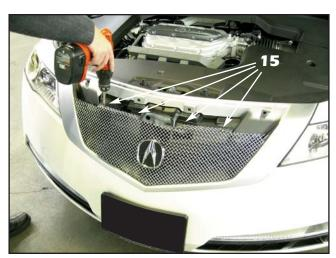
**15**. Reinstall the mesh section using the #8 x 1/2" black truss head screws, making sure it is tight against the foam tape installed in **Step 12**.
