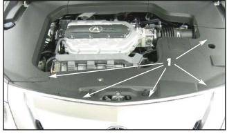
1. Remove the engine bay shroud by lifting straight up to release the clips and remove the cover (to be reinstalled).
