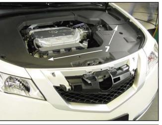
Reinstall the engine bay shroud removed in Step 1 using the factory push pins.
