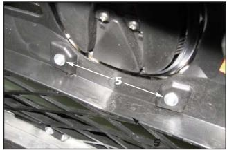
Once the eight (8) factory torx screws are removed, pull the grille insert forward and remove it from the grille surround.
