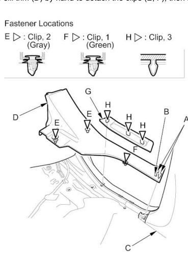
3. If necessary, pull up the rear side outer trim (G) to detach the clips (H), then remove the trim.
