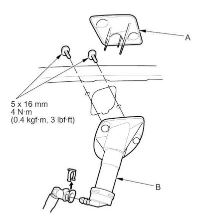
3. Install the nozzle in the reverse order of removal. Take care not to pinch the washer tube. Check the headlight washer operation.
