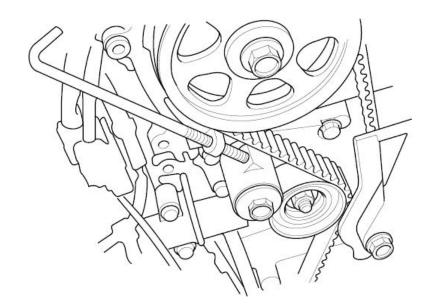
14. Remove the timing belt guide plate (A).
