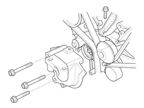
16. Remove the idler pulley bolt (A) and the idler pulley (B), then remove the timing belt. Discard the idler pulley bolt.
