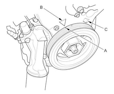
3. Check that the No. 1 piston top dead center (TDC) mark (A) on the front camshaft pulley and the pointer (B) on the front upper cover are aligned.
