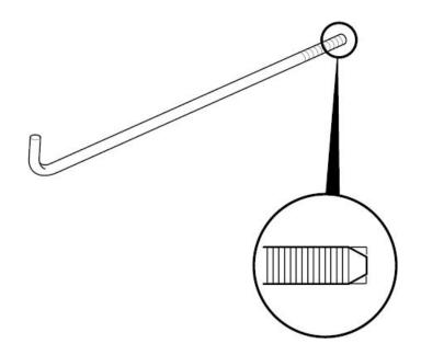
13. Thread the battery clamp bolt in as shown to hold the timing belt adjuster in its current position. Tighten it by hand, do not use a wrench.
