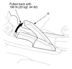
2. If the number of lever clicks is not as specified, adjust the parking brake. NOTE: Minor parking brake lever adjustments (1 to 2 clicks) can be made with the adjusting nut (see parking brake minor adjustment). If a larger adjustment is required, follow the major adjustment procedure using the adjuster nut at the parking brake drum (see parking brake major adjustment).
