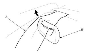
4. Remove the bolts from the base of the seat-back (A).
