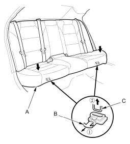
2. Remove the seat cushion (A), and release the center seat belt buckles (B) from the slits (C).
