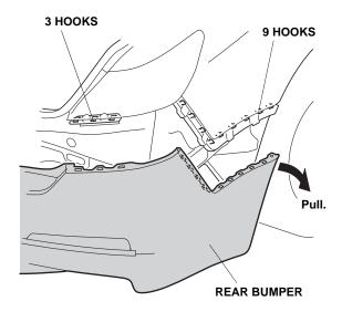
With the help from an assistant, remove the rear bumper (four hooks, and unplug the two vehicle connectors). Place the rear bumper on a blanket to prevent damage.
