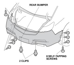
• On each side, release the 12 hooks, and gently pull the rear bumper out from the body.
