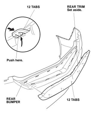
3. Install the rear sport trim to the rear bumper. Make sure all the tabs are properly snapped in place.
