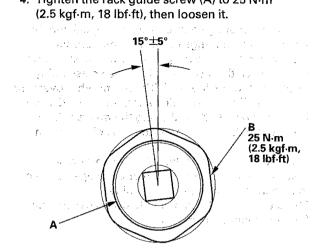
Retighten the rack guide screw to 3.9 N·m (0.4 kgf·m, 4 lbf·ft), then back it off to the specified angle.
