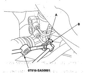
3. Remove the old sealant from the rack guide screw (A), and apply new sealant (Three Bond 1215 or Loctite 5699) to the middle of the threads (B). Loosely install the rack guide screw on the steering gearbox.
