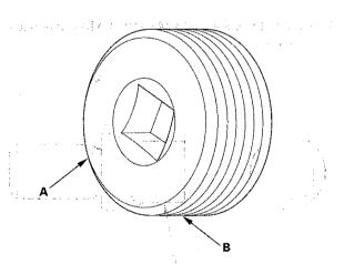
4. Tighten the rack guide screw (A) to 25 N·m
