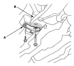
Lower the jack supporting the front suspension subframe (A) with the special tool slowly until the front suspension subframe has dropped about 50 mm (1 15/16 in.).
