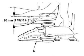
22. Remove the P/S heat baffle plate (A).
