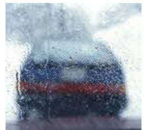
Impaired view from worn wiper blades
