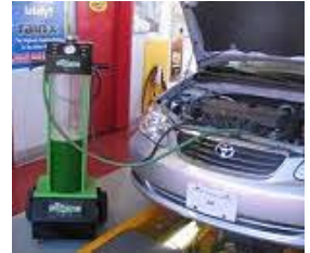
Coolant flush equipment
