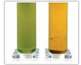
Clean vs. dirty, acidic coolant (antifreeze)
