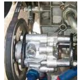
New power steering pump installed
