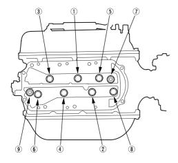
3. Install the upper cover. Tighten the bolts and nuts sequentially in two or three steps. Always use a new intake manifold gasket (2002-2004 Models).
