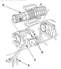
3. Remove the vacuum hose(s) (B) and breather pipe (C), then remove the intake air duct (D).
