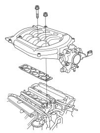
11. Remove the upper cover (A), then remove the intake manifold (B) and spacer (C) (2002-2004 models).
