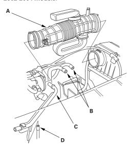
11. Install the EVAP canister hose (D) (1999-2001 models) or vacuum hose (D) (2002-2004 models).
