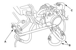
5. Install the EVAP canister hose (C) (2002-2004 models).
