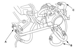
9. Remove the EVAP canister hose (C) (2002-2004 models).
