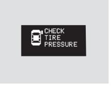
Each tire has its own pressure sensor. If the air pressure of a tire becomes significantly low, the sensor in that tire immediately sends a signal that causes the low tire pressure indicator in the instrument panel to come on. If this happens, you will see which tire is losing the pressure in the multi-information display along with a "CHECK TIRE PRESSURE" message.
