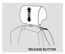
All head restraints adjust for height. The tilt of the front head restraints is also adjustable. You need both hands to adjust the restraint. Do not attempt to adjust it while driving. To raise it, pull upward. To lower the restraint, push the release button sideways, and push the restraint down. To adjust the tilt, pivot the front head restraint to the desired position.
