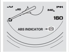
If this indicator comes on, the antilock function of the braking system has shut down. The brakes still work like a conventional system, but without anti-lock. You should have your dealer inspect your vehicle as soon as possible.
