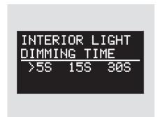
The interior lights fade out when you close all doors (see page 113). Select how long it takes for the interior lights to fade out (in seconds) from 5S, 15S, or 30S, and enter your selection by moving the pointer with the > side of the INFO button.
