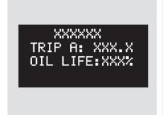
This shows the remaining life of the engine oil. It shows 100% after the engine oil is replaced and the display is reset. The engine oil life is calculated based on engine operating conditions and accumulated engine revolutions.
