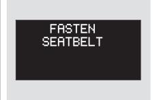
In addition to the seat belt reminder in the instrument panel, the multi-information display interrupts the current display and shows "FASTEN SEAT BELT" for about 6 seconds if you do not fasten your seat belt while driving. This message repeats if you ignore it and do not wear your seat belt while the vehicle is moving.
