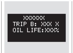
The remaining engine oil life is displayed on the multi-information display as a percentage when you turn the ignition switch to the ON (II) position.
