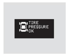
Your vehicle is equipped with a tire pressure monitoring system (TPMS) that turns on every time you start the engine and monitors the pressure in your tires while driving.
