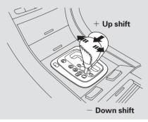
When you accelerate away from a stop, the transmission will start in first gear and then automatically upshift to second gear. You have to manually upshift between second and fifth gears. Make sure you upshift before the engine speed reaches the tachometer's red zone. The transmission remains in the selected gear (5, 4, 3). There is no automatic downshift when you push the accelerator pedal to the floor.
