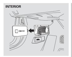
The vehicle's fuses are contained in two fuse boxes. The interior fuse box is on the driver's lower left side. To remove the fuse box lid, put your finger in the notch on the lid, pull it toward you, and take it out of its hinges.
