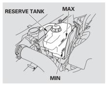
Look at the coolant level in the radiator reserve tank. Make sure it is between the MAX and MIN lines. If it is below the MIN line, see **Adding Engine Coolant** on page 221 for information on adding the proper coolant.
