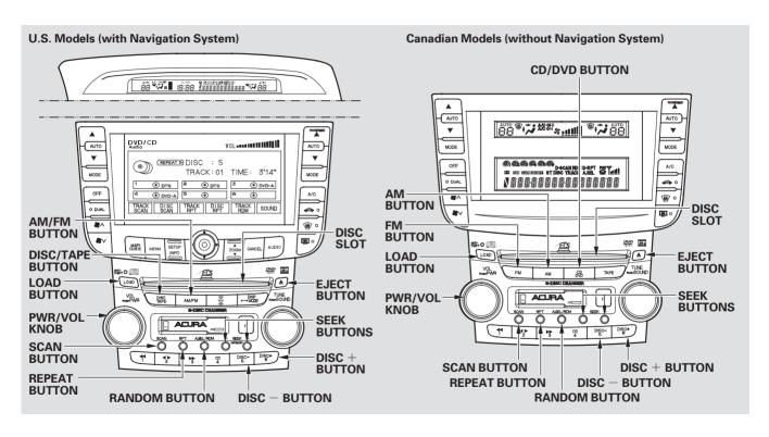
Your vehicle's audio system has an in-dash disc changer that holds up to six discs. You operate this disc changer with the same controls used for the radio. To operate the disc changer, the ignition switch must be in the ACCESSORY (I) or ON (II) position.
