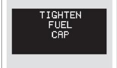
If the fuel fill cap is missing or not tightened properly, you will see "TIGHTEN FUEL CAP". Make sure the fuel cap is installed and tightened properly at least once.
