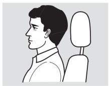
Adjust the driver's head restraint so the back of your head rests against the center of the restraint.
