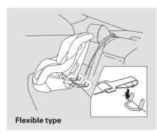
Other LATCH-compatible seats have a flexible-type connector as shown above.
