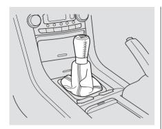
The manual transmission is synchronized in all forward gears for smooth operation. It has a lockout so you cannot accidentally shift from fifth to reverse instead of sixth (see page 191). When shifting up or down, make sure you push the clutch pedal down all the way, shift to the next gear, and let the pedal up gradually. When you are not shifting, do not rest your foot on the clutch pedal. This can cause your clutch to wear out faster.
