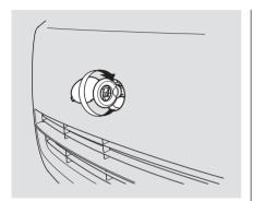
4. Screw the towing hook into the hook extension, and tighten it securely by hand.
