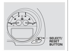
To reset a trip meter, display it, then press and hold the Select/Reset button until the number resets to "0.0."
