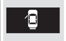
If the trunk or any door is not closed tightly, the display reminds you to close the open trunk or the door(s) before you start driving.
