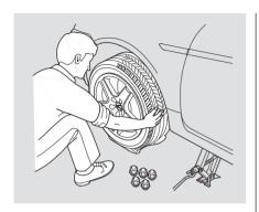
9. Remove the wheel nuts, then remove the flat tire. Temporarily place the flat tire on the ground with the outside surface of the wheel facing up. You could scratch the wheel if you put it face down.
