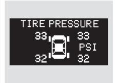
To see the inflation pressure of all four tires, press the SEL/RESET button. The display changes as shown above.
