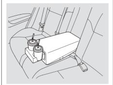
The rear beverage holder is in the rear seat armrest. Open the beverage holder by pushing the front of it, and pulling the holder all the way out.
