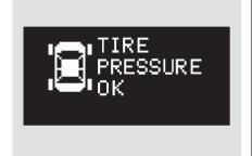
When you press the > side of the INFO button three times after you turn the ignition switch to the ON (II) position, you will see the above display.
