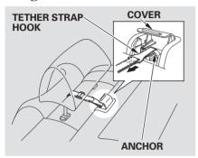
1. After properly securing the child seat (see page 46), lift the head restraint, then route the tether strap over the seat-back and through the legs of the head restraint.
