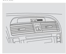
On models without Navigation System The clock displays the time with the ignition switch in the ON (II) position. If your vehicle's battery is disconnected or goes dead, you will need to reset the clock.
