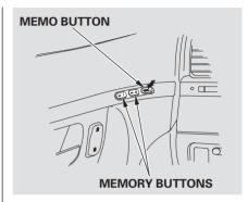
3. Press and release the MEMO button on the driver's door. You will hear a beep. Immediately press and hold one of the memory buttons (1 or 2) until you hear two beeps. The indicator in the memory button will come on. The current positions of the driver's seat and outside mirrors are now stored.
