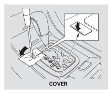
3. Put a cloth on the edge of the shift lock release slot cover. Using a small flat-tipped screwdriver or a metal fingernail file, carefully pry on the edge of the cover to remove it.
