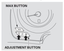
Adjust the brightness of the instrument panel by pressing the — or + side of the adjustment button. Press + to increase the brightness and — to decrease it. You can adjust the brightness with the headlight switch on or off.
