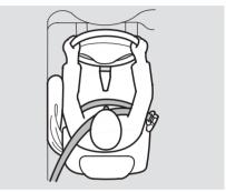
If you ever have a moderate to severe side impact, sensors will detect rapid deceleration and signal the control unit to instantly inflate either the driver's or the passenger's side airbag.
