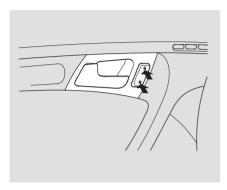
Each front door has a master door lock switch. Either switch locks and unlocks all doors. Push the bottom of the switch to lock the doors and the top to unlock them.
