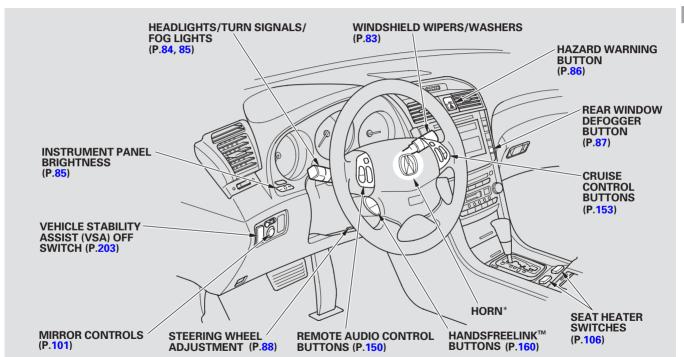
$oldsymbol{*}$ : To use the horn, press the center pad of the steering wheel.
