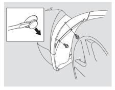
1. Start the engine. If you are replacing a driver's side bulb, turn the steering wheel all the way to the right. If you are replacing a passenger's side bulb, turn the steering wheel to the left. Turn off the engine.
