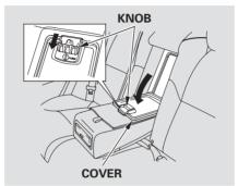
The trunk pass-through cover can be opened from either side; it folds forward onto the center armrest. Open the cover by sliding the knob downward and pushing or pulling on the cover. To close the cover, swing it up and push firmly on the top. Make sure it latches properly.
