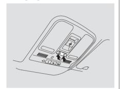
The front ceiling light has a three-position switch; ON, Door Activated, and OFF.
