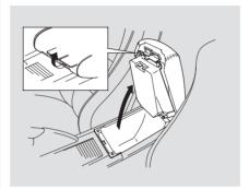
To open the console compartment, pull up on the right lever, and lift the armrest. To open the console compartment storage area, pull up on the left lever, and lift the armrest. To close, lower the armrest, and push it down until it latches.
