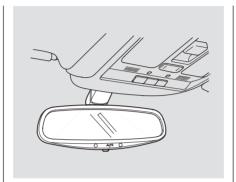
The inside mirror can automatically darken to reduce glare. To turn on this feature, press the button on the bottom of the mirror. The AUTO indicator comes on as a reminder. When it is on, the mirror darkens when it senses the headlights of a vehicle behind you, then returns to normal visibility when the lights are gone. Press the button again to turn off this sensing.
