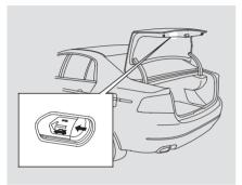
As a safety feature, your vehicle has a release lever on the trunk latch so the trunk can be opened from inside. To open the trunk, push the release lever to the left.
