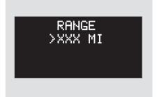
When the display shows the initial trip computer screen, press the > side of the INFO button to display "RANGE". This is the estimated distance you can travel on the fuel remaining in the tank. This distance is estimated from the fuel economy you received over the last several miles, so it will vary with changes in speed, traffic, etc.
