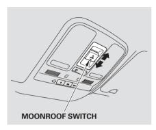
To slide the moonroof open, pull back the moonroof switch firmly. The moonroof automatically opens all the way. To stop the moonroof from opening fully, push the switch forward briefly.
