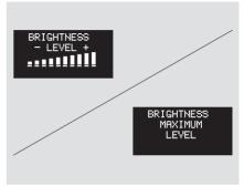
To reduce glare at night, the instrument panel illumination dims when you turn the light switch to ₹005 or ₹00 . Pressing the MAX button will bring it to the maximum level.
