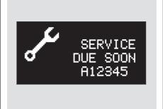
When the engine oil life reaches 15 percent, the display shows "SERVICE DUE SOON" and the code for the maintenance items to be performed.
