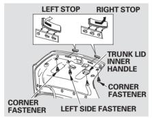
1 a. Determine which back-up light is out (left or right), then open the trunk.
