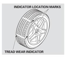
Your vehicle's tires have wear indicators molded into the tread. When the tread wears down to that point, you will see a 1/2 inch (12.7 mm) wide band running across the tread. This shows there is less than 1/16 inch (1.6 mm) of tread left on the tire. A tire that is this worn gives very little traction on wet roads. You should replace the tire if you can see the tread wear indicator in three or more places around the tire.
