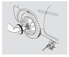
11. Put on the spare tire. Put the wheel nuts back on finger-tight, then tighten them in a crisscross pattern with the wheel nut wrench until the wheel is firmly against the hub. Do not try to tighten them fully.
