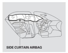
In a moderate to severe side impact, sensors will detect rapid deceleration and signal the control unit to instantly inflate the side curtain airbag on the driver's or the passenger's side of the vehicle.
