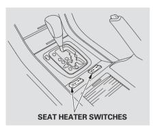
Both front seats are equipped with seat heaters. The passenger seat only has heaters in the seat bottom because of the side airbag system. The ignition switch must be in the ON (II) position to use them. Push the HI side of the switch to rapidly heat up the seat. After the seat reaches a comfortable temperature, push the LO side of the switch. This will keep the seat warm.
