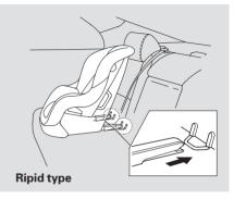
3. Place the child seat on the vehicle seat, then attach the seat to the lower anchors according to the child seat maker's instructions.
