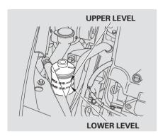
Check the level on the side of the reservoir when the engine is cold, and the engine compartment right-side cover is off (see page 217). The fluid should be between the UPPER LEVEL and LOWER LEVEL. If not, add power steering fluid to the UPPER LEVEL mark.
