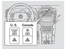
This indicator alerts you that the passenger's front airbag has shut off because weight sensors detect the weight of an infant or small child on the front passenger's seat. It does not mean there is a problem with the airbag.
