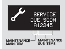
When the remaining engine oil life is 15%, you will see the message "SERVICE DUE SOON" along with all maintenance items that are needed at oil change time. Refer to page 213 for a complete list of the maintenance main items and sub items.
