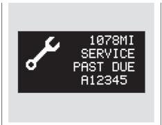
If the indicated maintenance service is not done and the remaining engine oil life gets less than 0%, you will see the message "SERVICE PAST DUE" on the display. Immediately have the service performed, and make sure to reset the display as previously described.
