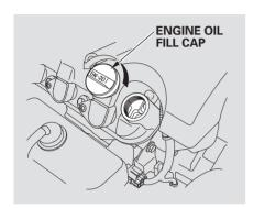
Unscrew and remove the engine oil fill cap on top of the valve cover. Pour in the oil slowly and carefully so you do not spill. Clean up any spills immediately. Spilled oil could damage components in the engine compartment. Install the engine oil fill cap, and tighten it securely. Wait a few minutes, and recheck the oil level (see page 179). Do not fill above the upper mark; you could damage the engine.
