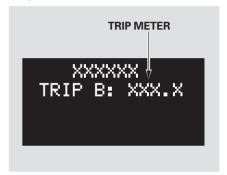
This meter show the number of miles (U.S.) or kilometers (Canada) driven since you last reset it. There are two trip meters: Trip A and Trip B. When you first turn the ignition switch to ON (II), Trip A is displayed. Switch between Trip A and Trip B by pressing the Select/Reset button repeatedly. Each trip meter works independently, so you can keep track of two different distances
