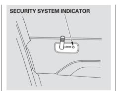
Once the security system is set, opening any door or the hood without using the key or the remote transmitter will cause the system to alarm. It also alarms if the radio is removed from the dashboard or the wiring is cut.
