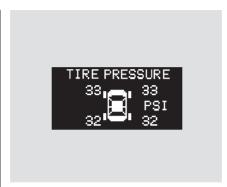
To see the inflation pressures of all four tires, press the SEL/RESET button. The display changes as shown above.
