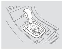
To shift from any position, press firmly on the brake pedal. You cannot shift out of Park when the ignition switch is in the LOCK (0) or ACCESSORY (I) position.
