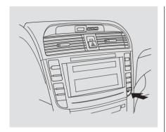
The rear window defogger clears fog, frost, and thin ice from the window. Push the defogger button to turn it on and off. The indicator in the button comes on to show the defogger is on. If you do not turn it off, the defogger will shut itself off after about 15 minutes. It also shuts off when you turn off the ignition. You have to turn it on again when you restart the vehicle.
