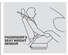
The passenger's advanced front airbag system has weight sensors under the seat. Although we do not encourage carrying an infant or small child in the front passenger's seat, if the sensors detect the weight of an infant or small child, the system will automatically turn the passenger's front airbag off.
