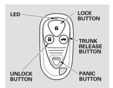
LOCK — Press this button once to lock all doors. Some exterior lights will flash. When you push LOCK twice within 5 seconds, you will hear a beep to verify that the doors are locked and the security system has set. You cannot lock the doors if any door is not fully closed or if the key is in the ignition switch.
