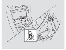
There are two accessory power sockets. One is in the front of the center console under the utility pocket lid. The other is under the armrest in the console compartment storage area.
