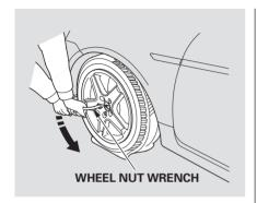
6. Loosen each wheel nut 1/2 turn with the wheel nut wrench.
