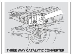
A defective three way catalytic converter contributes to air pollution, and can impair your engine's performance. Follow these guidelines to protect your vehicle's three way catalytic converter.
