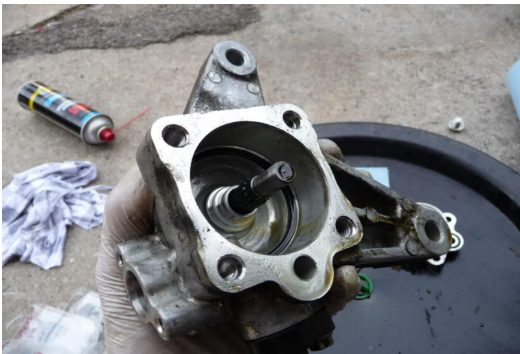
8c. Turn it around and hammer the shaft out.
