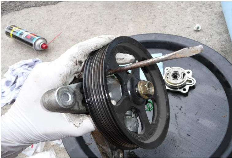
8b. Take out the C-Clip using your Snap Ring Pliers .
