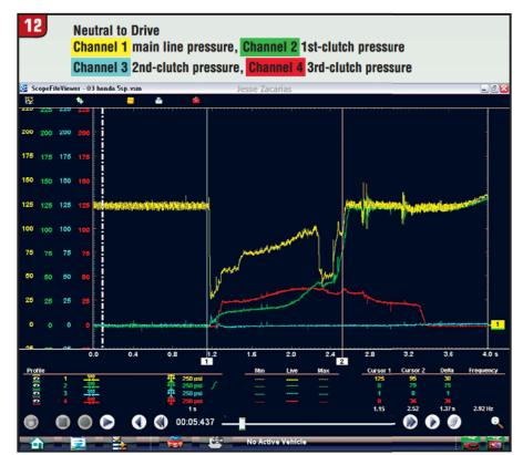
from Neutral to Drive (Figure 12) and it requires only 36 psi to engage, we can imagine what 50 psi can do with the second clutch on with up to 130 psi. When these vehicles are being driven in fourth gear, it also does not take much throttle increase to get a downshift to second. On my many road tests on this car, 4-2 downshift was a normal shift when I entered the freeway.
