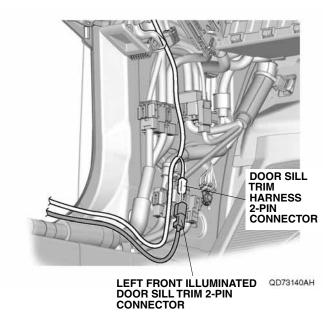
60. Position the left front illuminated door sill trim to the vehicle panel as shown.
