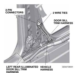
67. Position the left rear illuminated door sill trim to the vehicle panel as shown.
