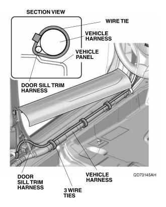
65. Plug the door sill trim harness 2-pin connector into the left rear illuminated door sill trim 2-pin connector.
