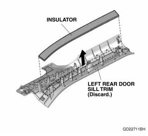
30. Align the edge of the insulator with the rib on the left rear illuminated door sill trim.
