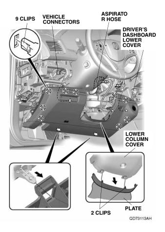
18. Turn the knob, and remove the driver's dashboard under cover and unplug the vehicle connector.
