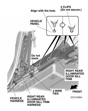
55. Secure the right rear illuminated door sill trim harness to the vehicle harness with two wire ties.
