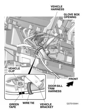
45. Secure the door sill trim harness to the vehicle harness with two wire ties.
