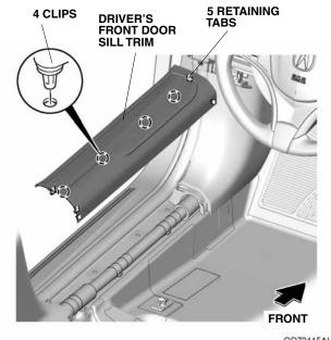
20. Pull away the door opening seal, and remove the driver's kick panel.
