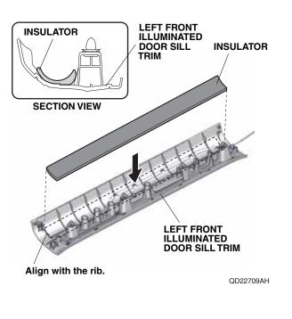
27. Using isopropyl alcohol on a shop towel, thoroughly clean the left front illuminated door sill trim where the aluminum tape will attach.
