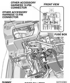
DUMMY CONNECTOR (Discard.) DOOR SILL TRIM HARNESS 12-PIN CONNECTOR 38. Secure the door sill trim harness to the vehicle harness with two wire ties.
