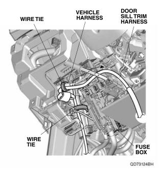
39. Route the door sill trim harness as shown. Align the green tape on the door sill trim harness with the vehicle harness as shown, and secure the door sill trim harness to the vehicle harness with one wire tie.
