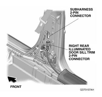
53. Secure the subharness and 2-pin connectors to the vehicle harness with two wire ties.
