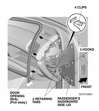
9. Remove the passenger's dashboard upper cover and unplug the vehicle connector.
