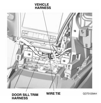
44. Align the green tape on the door sill trim harness with the vehicle clip, and secure the door sill trim harness to the vehicle harness with one wire tie.
