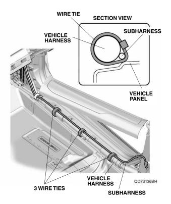
52. Plug the subharness 2-pin connectors into the right rear illuminated door sill trim 2-pin connector.
