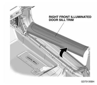
51. Secure the subharness to the vehicle harness with three wire ties.
