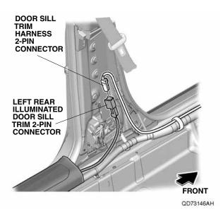
66. Secure the door sill trim harness, left rear illuminated door sill trim harness, and 2-pin connectors to the vehicle harness with two wire ties.
