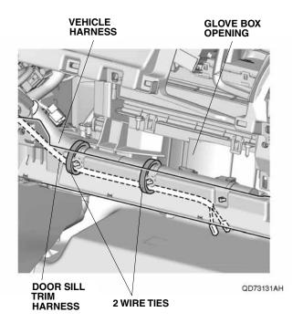
46. Plug the two door sill trim harness 2-pin connectors into the right front illuminated door sill trim 2-pin connector and subharness 2-pin connector.
