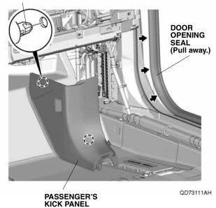
16. Pull away the door opening seal, and remove the driver's dashboard side lid.
