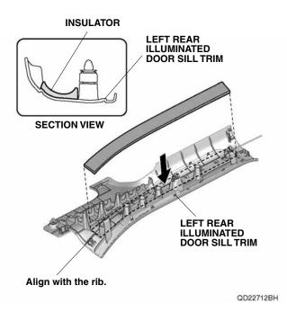
31. Using isopropyl alcohol on a shop towel, thoroughly clean the left rear illuminated door sill trim where the aluminum tape will attach.
