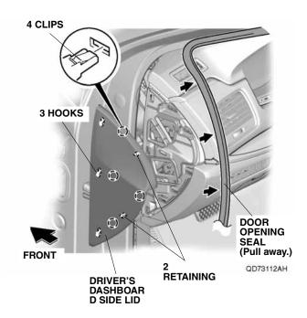
17. Remove the driver's dashboard lower cover. Unplug the vehicle connectors and aspirator hose, then remove the plate.
