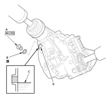
2. Make sure the transfer assembly fluid level is at the proper level (C).
