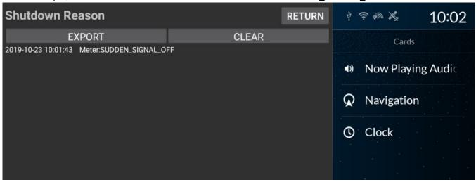
There was a complete loss of signal on the network between the meter (gauge control module) and the previous transmitting unit on the network. In this example, the previous unit is the tuner unit. Although the specific cause is not identified, the failure was confirmed and the components and connections that should be inspected have been isolated.
