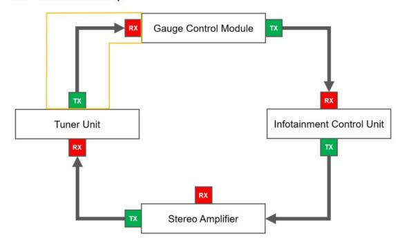
Refer to the specific model and trim information in the Audio and Visual System MOST Bus Diagnostics Mode section in the service information to determine each control unit's location on the network and identify where a failure potentially occurred.
