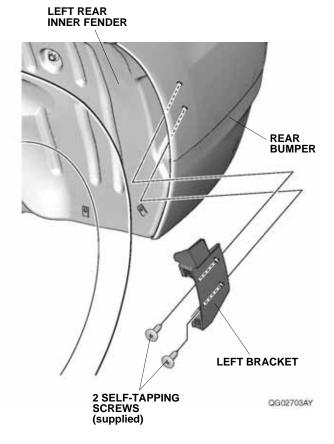
14. Loosely install the left rear splash guard to the left bracket and left rear inner fender with the four self-tapping screws supplied.
