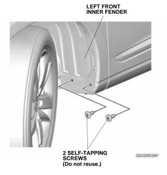
4. Loosely install the left front splash guard to the left front inner fender with the four self-tapping screws supplied.
