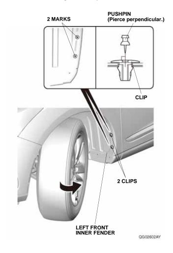
2. Using a pushpin, pierce the center of the two clips on the left front inner fender.
