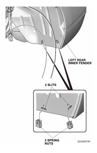
11. Peel back the left rear inner fender, and remove the spring nut.
