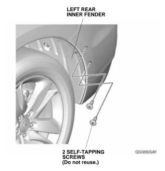
8. Using a pushpin, pierce the center of the two dimples in the left rear inner fender.
