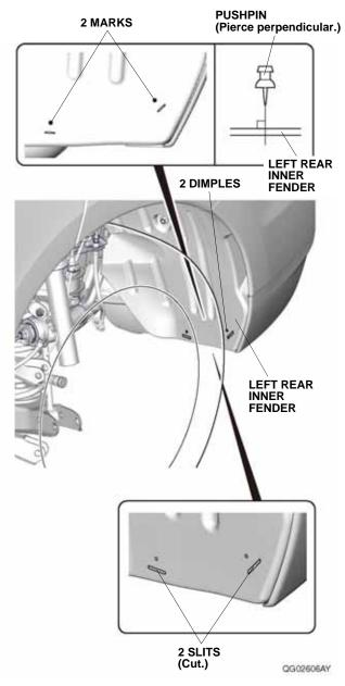
9. Using a utility knife, cut the two slits in the left rear inner fender.
