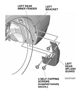
15. Loosely secure the left rear splash guard to the rear bumper with the self-tapping screw supplied.
