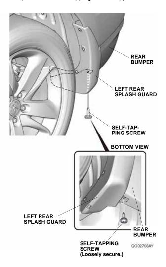
16. While holding the left rear splash guard against the rear bumper and left rear inner fender, tighten the four self-tapping screws in the order shown. NOTE: Make sure there are no gaps between the left rear splash guard and the vehicle body. If there is a gap, loosen the self-tapping screws, hold the splash guard against the body, and tighten the screws.
