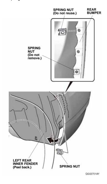
12. Install one spring nut to the rear bumper as shown. NOTE: Make sure you install the spring nut in the correct position and with the large hole facing out.
