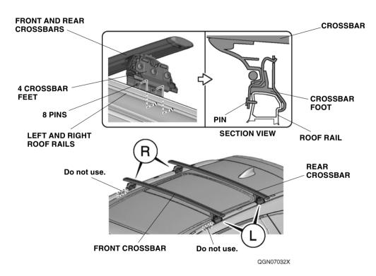
To line up the crossbar pins with the roof rails, you may need to slightly loosen the crossbar screws. Make sure each clamp is fully seated on the roof rail as shown. Loosely tighten each screw, then torque them to 3.0 lb-ft  $(4 \text{ N} \cdot \text{m})$ .
