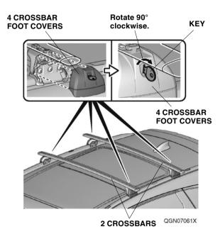
Make sure the crossbars are firmly secured by applying pressure to them as shown. Store the keys and special tool in a safe place.
