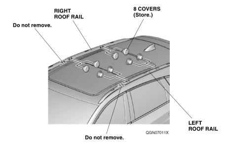
On each crossbar foot, turn the supplied key 90° counterclockwise to unlock the cover. Then, remove them. Identify the front and rear crossbar by their shapes shown.
