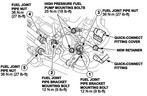
23. Tighten the fuel joint pipe bracket mounting bolts and the fuel joint pipe nuts to the specified torque in the numbered sequence shown.
