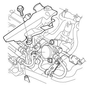
5. Remove the quick-connect fitting cover.
