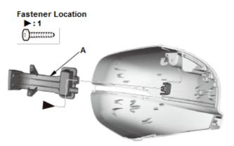
6. Remove the screw with a TORX T15 bit, and then remove the side turn light (A). (for some models)
