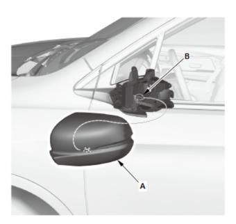
5. Remove the mirror housing cover (A), and then disconnect the connector (B). (for some models)
