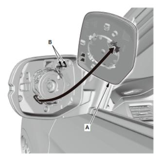
4. Remove the mirror holder (A), and then disconnect the connectors (B).
