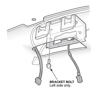
6. Slide the transceiver bracket onto the transceiver.
