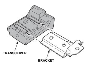
7. Connect the black and green connector into the transceiver. Then install the clip on the connector into the hole in the bracket.
