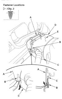
Turn the steering wheel to the left, and release the left tab (A) of the upper column cover (B) while pushing on the lower column cover (C) from the front.
