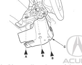
Install the upper and lower column covers in the reverse order of removal, and push the hooks into place securely.
