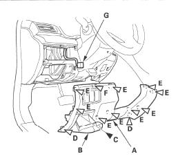
3. Disconnect the VSA OFF switch connector (G).
