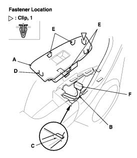
6. Remove the screw securing the door panel (A).
