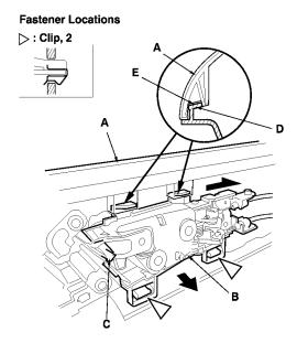
While holding the door panel (A) away from the door, disconnect the courtesy light bulb socket (B).
