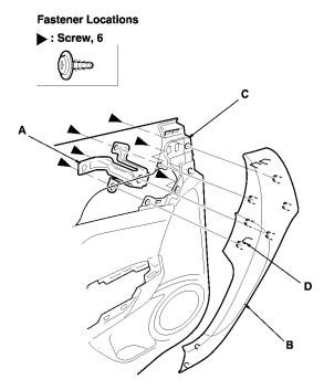
15. Remove the screw, and release the tabs (A), then remove the grip base (B) from the grip cover (C).
