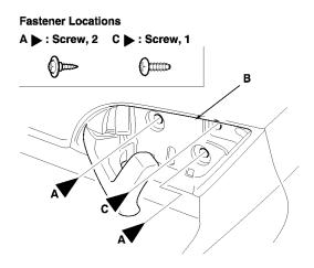
Release the hooks (A), and remove the pull pocket cap (B), then remove the screw.
