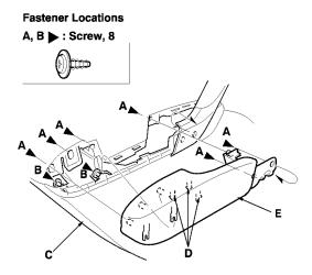
13. Remove the screw, then remove the grip bracket B. Release the hook (A), then remove the door pull pocket (C) from the armrest (D).
