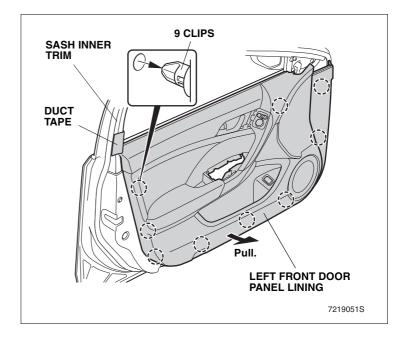
14. Lift the left front door panel lining upward to release the two tabs from the inner handle case.
