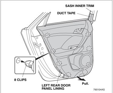
36. Lift the left rear door panel lining upward to release the two tabs from the inner handle case.
