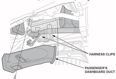
17.4. Connect the dashboard wire harness 4P connector to the front passenger's airbag, then reinstall the glove box.
