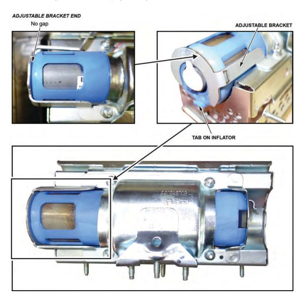
13. Hold the bracket against the inflator, then install the new 5 mm locknuts and torque them in sequence to **3.9 N•m** (**34 lb-in**).
