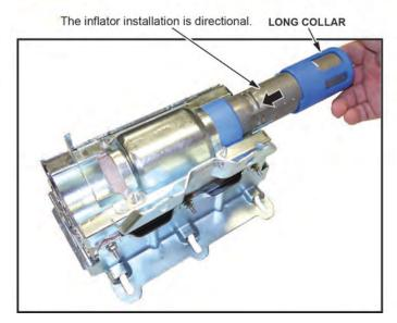
12.2. Slide the inflator in until the plastic collar contacts the bracket. The two tabs should align with the side of the airbag module and the metal tab as shown. There should be no space or gap between the inflator and bracket.
