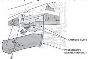
3.4. Remove the mounting nuts and the mounting bolts. Release the hooks of the hook plate and remove it.
