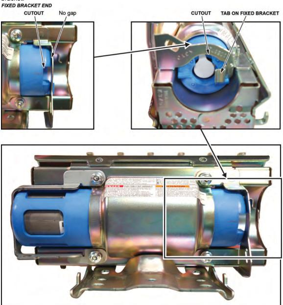
12.3. Install the bracket included in the kit onto the airbag module. Check there is no space or gap between the inflator and bracket by pushing the bracket against the inflator.
