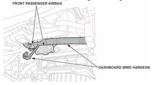
3.3. Remove the passenger's dashboard duct, then detach the harness clips.
