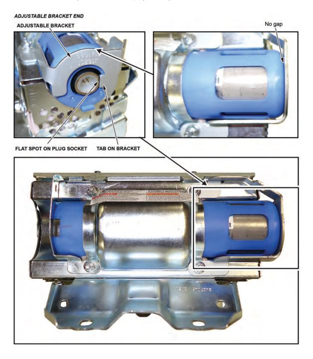
13. Hold the bracket against the inflator, then install the new 5 mm locknuts and torque them in sequence to **3.9 N•m** (**34 lb-in**).
