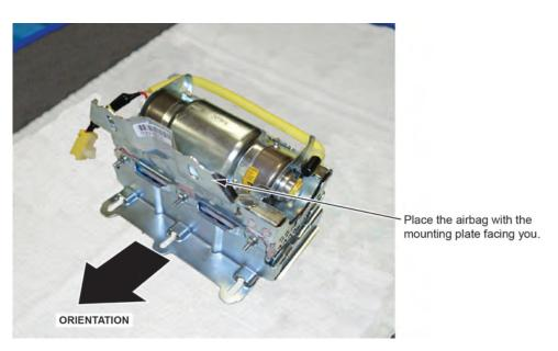
5. Visually inspect the airbag and the inflator for any unusual writing or markings. Refer to IDENTIFYING COUNTERFEIT AIRBAGS.
