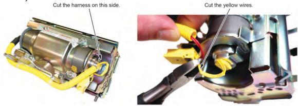
8.2. Strip away about 1 inch of the yellow wire insulation, then twist the wires together.
