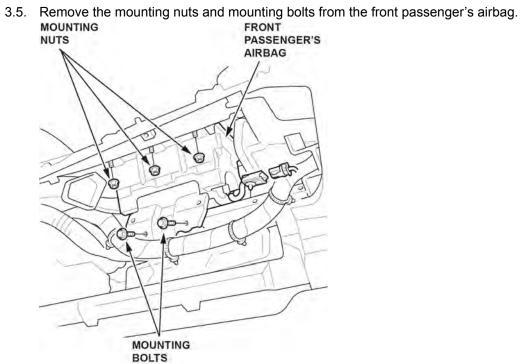
3.6. Release the pin and remove the front passenger's airbag.
