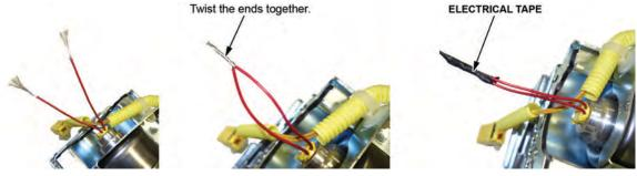
8.3. Tape the twisted ends with electrical tape.
