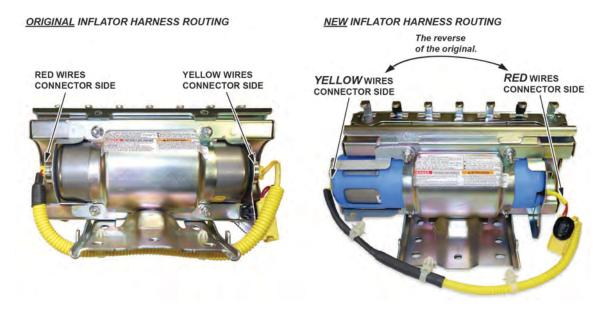
15.2. Connect the red wire connector to the connector on the side with the short plastic collar. Align the "T" shape in the inflator harness connector with the T-shaped inflator connector, then press the connector into place.
