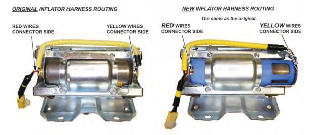
15.2. Connect the red wire connector to the connector on the side with the short plastic collar. Align the "T" shape in the inflator harness connector with the T-shaped inflator connector, then press the connector into place.
