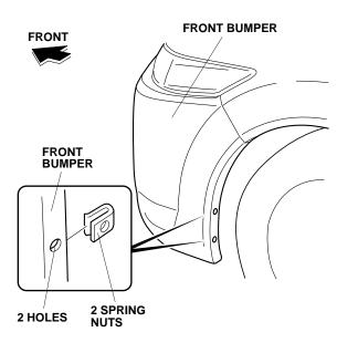
4. Install three clip nuts to the bottom of the front bumper as shown.
