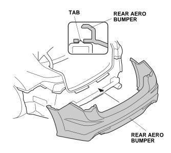
9. Secure the rear aero bumper to the vehicle by reusing the two bolts, ten self-tapping screws, two clips, and the two caps.
