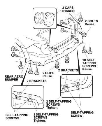
10. Tighten the two self-tapping screws installed in step 7.
