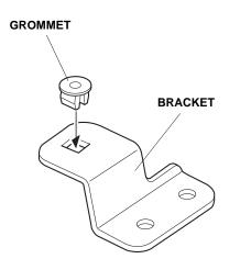
Loosely install two brackets on the left side of the rear aero bumper using two self-tapping screws. Install two brackets to the right side of the aero bumper the same way.
