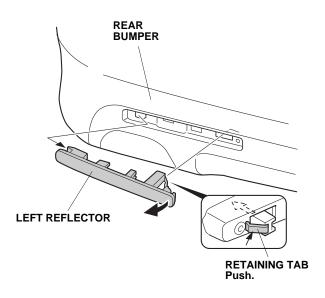
5. Transfer the left and right reflectors to the new aero bumper.
