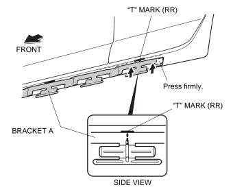
10. Detach the front end of the side lower bracket where you lightly pressed in step 8. Keep holding the end of the bracket. Reposition the top of the bracket to the top of the "T" mark (FR), and press on the front of the bracket firmly to adhere.
