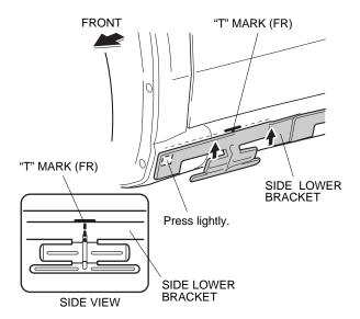
Raise the rear of the side lower bracket to contact the top of the "T" mark (RR). Press on the rear of the bracket (where you removed the adhesive backing) firmly to adhere.
