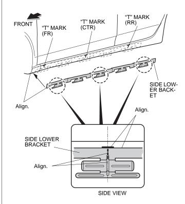
8. Raise the front of the side lower bracket to contact the top of the "T" mark (FR). Press on the front of the bracket (where you removed the adhesive backing) lightly to adhere.
