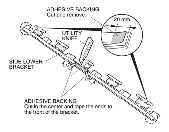
Using a utility knife, cut the adhesive backing in the center of the side lower bracket. Attach a piece of masking tape to each of the cut ends, and tape them to the front of the side lower bracket. 6. Using isopropyl alcohol on a shop towel, clean the area where the side under spoiler will attach.
