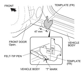
2. Position the template (marked CTR) on the vehicle body. Using a felt-tip pen, mark the vehicle body at the measurement shown.
