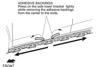
13. While wearing gloves, adhere the side lower bracket by firmly pressing on the double-sided tape. Take care not to press on the bracket mounting plates as it can deform the plates. The side under spoiler cannot be installed securely if the mounting plates are bent.
