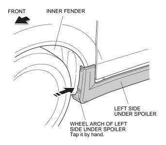
19. Loosely install the two 5 x 18 mm self-tapping screws into the two holes at the wheel arch of the left side under spoiler.
