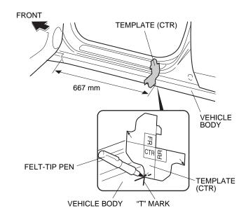
Open the left rear door. Position the template (marked RR) on the vehicle body. Using a felt-tip pen, mark the vehicle body at the measurement shown.
