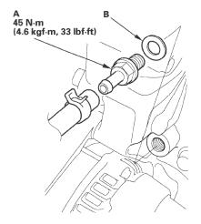
3. Install the parts in the reverse order of removal with a new washer (B).
