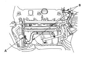
2. At idle, make sure there is a clicking sound from the PCV valve when the hose between the PCV valve and intake manifold is lightly pinched (A) with your fingers or pliers.
