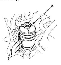
Raise the reservoir, then disconnect the return hose (A) to drain the reservoir. Take care not to spill the fluid on the body and parts. Wipe off any spilled fluid at once.
