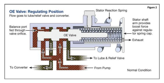
In many systems, a modest base line pressure is established by the PR springs, with higher pressures coming as a result of some demand-related boost system. As you can see in **Figure 2**, Honda does not use a conventional line pressure boost system. In the Honda system, more substantial PR springs and a stator load-related boost system establish a much higher base line pressure from the outset with modest boost increase at max pressure.
