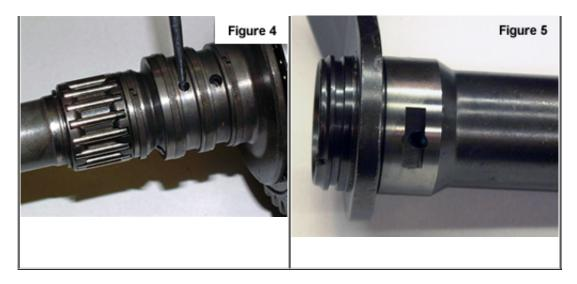
This circuit is generally fairly tight. The parallel circuit, on the other hand, does not have a positive seal where the stator support passes through the valve body (**Figure 5**).
