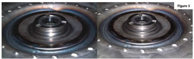
machined easily. **Figure 3** shows a turbine hub after the groove is cut (left), and the same hub with the late model seal installed (right).
