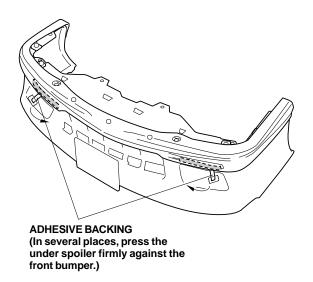
12. Reinstall the front grille, the front bumper and the front bulkhead cover. Make sure that all clips are installed securely.
