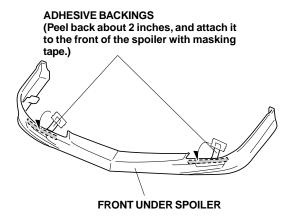
8. Using isopropyl alcohol on a shop towel, thoroughly clean the front bumper where the front under spoiler will be attached.
