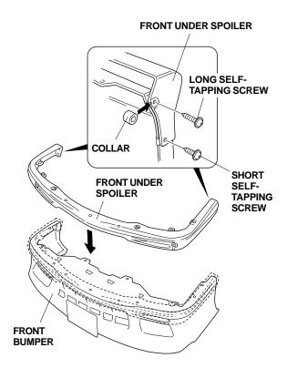
Position the front under spoiler on the front bumper, and install the two long and two short self-tapping screws with one collar on each side placed between the front under spoiler and the and front bumper. 10. Secure the front under spoiler to the front bumper with the three bumper bolts, six flange bolts, and nine flange nuts in the kit. Be careful not to mix up the bumper bolts with the flange bolts.
