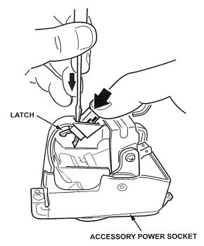
4. Insert a new latch into the accessory power socket.
