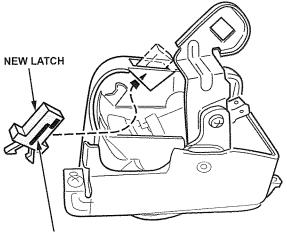
Make sure the slotted side of the latch is facing the open side of the power socket.
