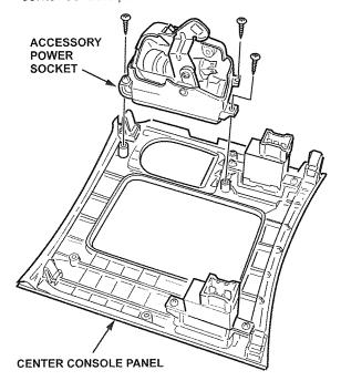
3. Remove the latch from the accessory power socket.
