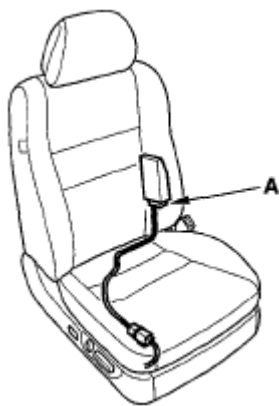
Fig. 336: Identifying OPDS Unit Harness 8P Connector Courtesy of AMERICAN HONDA MOTOR CO., INC.
