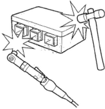
Fig. 9: Precaution - Do Not Bump (By Impact Wrench, Hammer, Etc.) Area Around SRS Unit Courtesy of AMERICAN HONDA MOTOR CO., INC.
