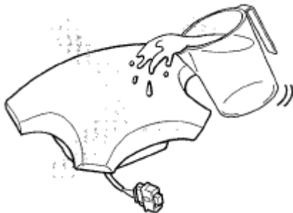
Fig. 5: Precaution - Keep Airbag Away From Any Oil, Grease, Detergent, Or Water Courtesy of AMERICAN HONDA MOTOR CO., INC.
