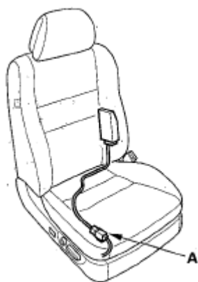
Fig. 333: Identifying Right Side OPDS Unit And 4P Connector Courtesy of AMERICAN HONDA MOTOR CO., INC.
