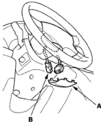
Fig. 396: Identifying Steering Wheel Access Panel And Airbag 4P Connector Courtesy of AMERICAN HONDA MOTOR CO., INC.
