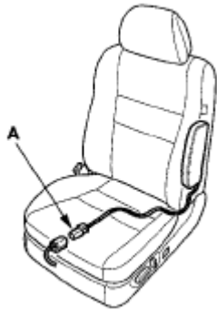
Fig. 398: Identifying Side Airbag 2P Connector Courtesy of AMERICAN HONDA MOTOR CO., INC.
