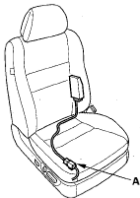
Fig. 331: Identifying Right Side OPDS Unit And 4P Connector Courtesy of AMERICAN HONDA MOTOR CO., INC.
