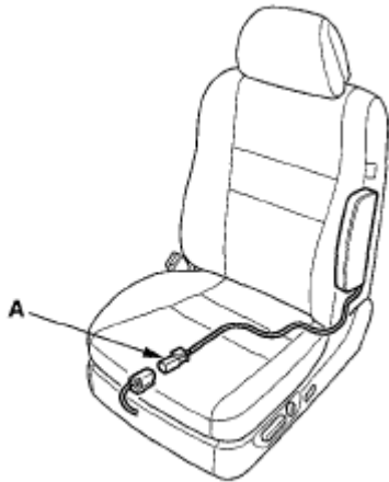
Fig. 30: Identifying Side Airbag 2P Connector Courtesy of AMERICAN HONDA MOTOR CO., INC.
