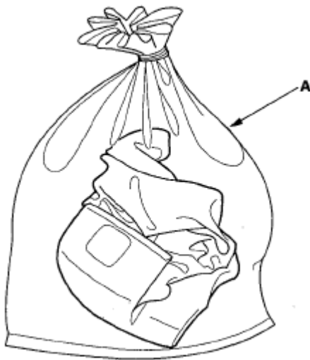
Fig. 402: Placing Airbag In Sturdy Plastic Bag Courtesy of AMERICAN HONDA MOTOR CO., INC.
