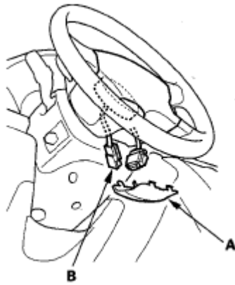
Fig. 378: Identifying Steering Wheel Access Panel And Airbag 4P Connector Courtesy of AMERICAN HONDA MOTOR CO., INC.
