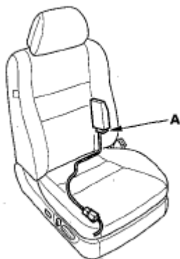
Fig. 324: Identifying OPDS Unit And 8P Connector Courtesy of AMERICAN HONDA MOTOR CO., INC.
