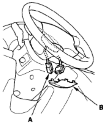
Fig. 381: Identifying Steering Wheel Access Panel And Airbag 4P Connector Courtesy of AMERICAN HONDA MOTOR CO., INC.
